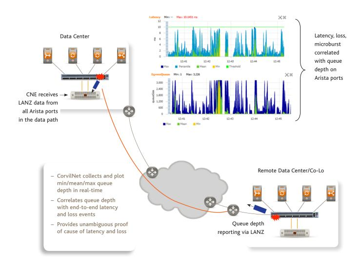
product path. In a single real-time view, CorvilNet enables the user to quickly correlate application performance issues with network latency, jitter and loss and any queuing congestion at an Arista port.
