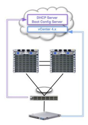
After the network stack is initialized, and an SVI created with the IP address specified in the DHCP response ToR-1 contacts the boot server specified in DHCP Option 67. ToR-1 downloads the appropriate start-up configuration or script based on the switch's unique identifier.
