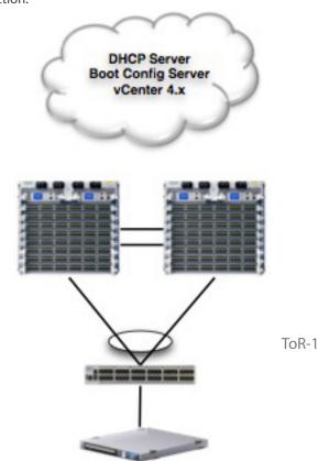
Once the switch is racked, connected, and powered on, ZTP takes care of the rest.
